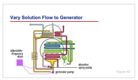
In more modern absorption chiller designs, **adjustable-frequency drives** (AFD), also known as variable-speed drives, are used to vary the speed of the generator pump motor, thus reducing the flow of solution to the generator. AFDs have the added benefit of saving pump energy at part-load conditions.
